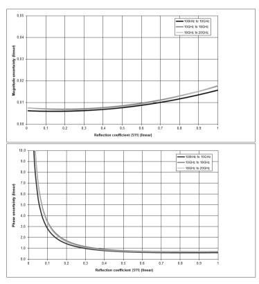
Typical accuracy of reflection magnitude and reflection phase measurements for the R&S®ZNBT20 in the frequency range from 100 kHz to 20 GHz, calibrated with a ZV-Z235 calibration kit that has been characterized with a DAkkS-accredited calibration
