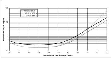
Typical accuracy of transmission magnitude and transmission phase measurements for the R&S®ZNBT8 in the frequency range from 9 kHz to 8.5 GHz. Analysis conditions:  $S_{11} = S_{22} = 0$ , cal. power –10 dBm, meas. power –10 dBm.
