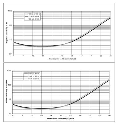
Typical accuracy of transmission magnitude and transmission phase measurements for the R&S®ZNBT20 in the frequency range from 100 kHz to 20 GHz. Analysis conditions:  $S_{11} = S_{22} = 0$ , cal. power –10 dBm, meas. power –10 dBm.
