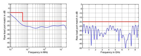
Raw load port match versus frequency for the R&S®ZNBT8.
