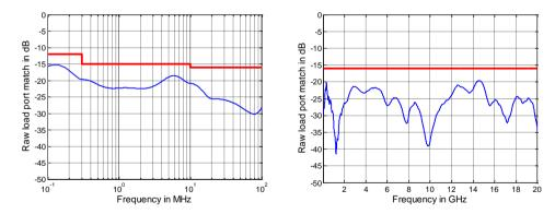
Raw load port match versus frequency for the R&S®ZNBT20.
