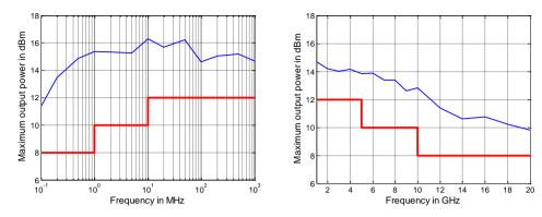
Maximum output power in dBm versus frequency for the R&S®ZNBT20.
