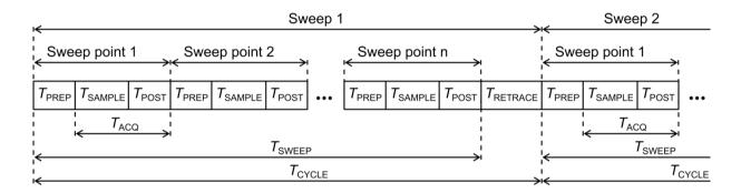
$T_{\mathsf{PREP}}$  Preparation time required to set up the internal hardware components
