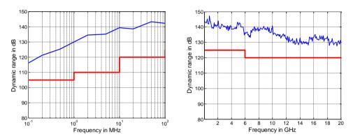
Dynamic range in dB versus frequency for the R&S®ZNBT20.
