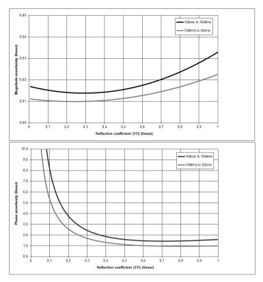
Typical accuracy of reflection magnitude and reflection phase measurements for the R&S $^{\otimes}$ ZNBT20 in the frequency range from 100 kHz to 20 GHz. Analysis conditions:  $S_{12} = S_{21} = 0$ , cal. power –10 dBm, meas. power –10 dBm.
