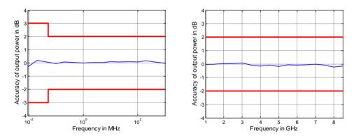
Output power accuracy in dB versus frequency for the R&S®ZNBT8.
