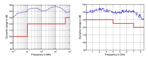
Dynamic range in dB versus frequency for the R&S®ZNBT8.
