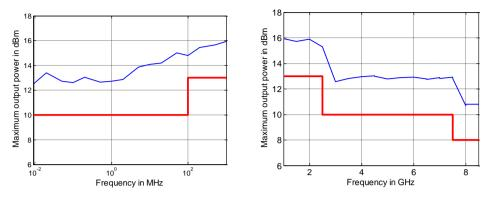
Maximum output power in dBm versus frequency for the R&S®ZNBT8.
